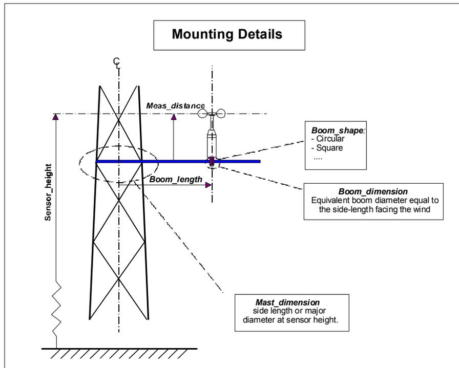
**Figure C-1: definition of mounting details.**
